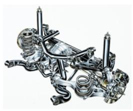
"One-dimensional cars don't The SVT Cobra independent rear suspension system has been re-tuned for the 2003 engine's higher torque output. fit the SVT philosophy," said John Coletti, chief engineer for Ford SVT, "and this is a very, very
