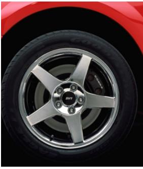
New cast-aluminum 17 x 9-inch wheels are fitted with 275/40ZR-17 Goodyear Eagle F1 tires. The braking system includes 13-inch Brembo<sup>TM</sup> front rotors with PBR<sup>TM</sup> dual-piston calipers, and 11.65-inch rear rotors with single-piston calipers. The pad material on the rear brakes has been upgraded for enhanced durability and brake performance.
