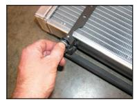
17. Install the lower bracket. It will mount just like it did on the factory unit. Install the 4 bolts and tighten.
