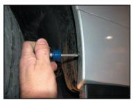
Remove the 2 bolts securing the P/S cooler and lower the cooler out of the way.
