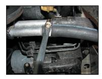
21. Attach the other end to the lower fitting on the heat exchanger. Install and tighten the clamp.
