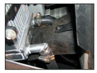
Install the black wire tie to prevent the lower hose from rubbing on the splash shield.
