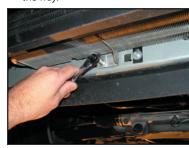
Remove the 4 bolts securing the factory heat exchanger to the front mounting brackets.
