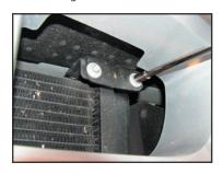
Move the assembly toward the radiator to unhook from the back of the bumper and gently lower to gain access to the hoses.
