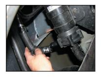
11. Disconnect the heat exchanger outlet hose from the engine. It is connected to a steel line just below the A/C compressor. You will disconnect the lower of the two hoses.
