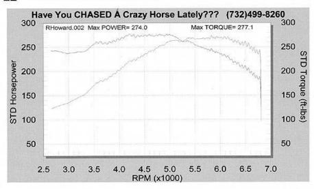
Here's the "before" dyno graph. No doubt, 274 <u>horsepower</u> from a stock Cobra is nothing to sneeze at, nor is 277 lbs.-ft. of torque. Obviously, the horsepower problems from '99 have been worked out.
