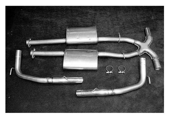
The FR500 kit comes complete with hangers, clamps, bolts, etc. The X-pipe aft of the mufflers cuts down on resonance and adds a bit of <u>torque</u>.
