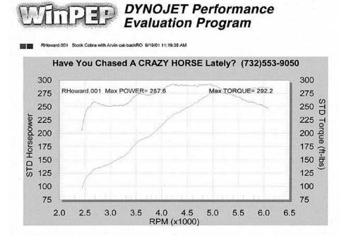
Of course, if 274 horsepower is good, 287.6 is a lot better. And look at that torque curve. We've never seen a <u>car</u> pick up 15 lbs.-ft. of torque from a cat-back system before.
