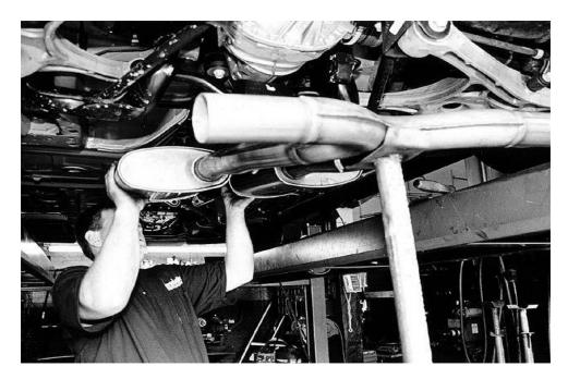
Using a pole jack to support the rear of the setup, O'Malley lined up the dual-mode mufflers to the factory H-pipe.
