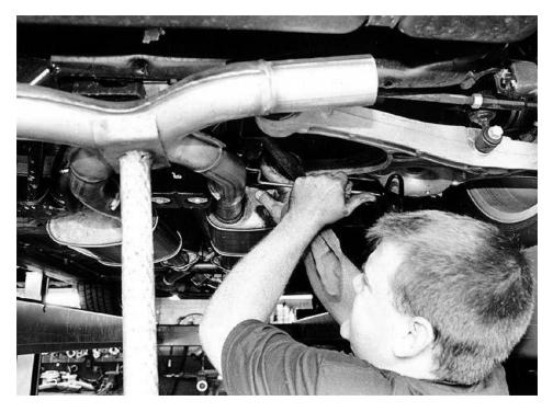
Check out the special whiz-bang tool specially designed for sliding steel hangers into rubber exhaust system mounts. You don't need one for the job, but O'Malley called it the greatest tool ever invented. He then slipped the tailpipe hanger in, but this turned out to be an incorrect move.
