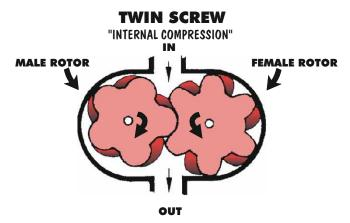
Air enters the supercharger through the rear or top rear and is "compressed" internally between the rotors. The male rotor rotates clockwise while the female rotor rotates counter clockwise trapping and compressing the air between them and then channeling ("screwing") the air toward the front where it is discharged. Note how the air is not pumped the long way around the rotors as with the Roots. The shortest smoothest path between two points is always best for optimum air flow.
