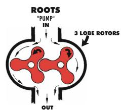
The Roots inlet air is caught by the rotors and then "pumped" circumferentially between the supercharger case and rotors and then discharged. All this surface area (rotors and case) coupled with the relatively long torturous air path creates more turbulence, friction, heat and pumping (HP) losses than the Twin Screw "compressor." Follow the air flow around the rotors and case and one can easily see why the Roots is clearly not as efficient as the Twin Screw
