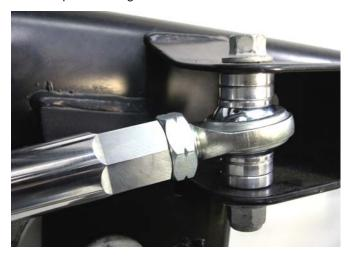
Note: MM recommends a spacer stack that is biased upwards (3 below, 1 above) as a starting inner-spacer configuration for **2003-04 IRS** cars. Place the OEM Spacer on the top of the MM spacer stack (OEM Spacer not shown in photo).
