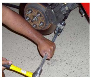
Remove the bolt securing the inner tie-rod end to the IRS sub-frame and remove the factory tie-rod from the vehicle.
