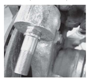
12. Slip the .060" thick spacer onto the bottom of the tapered stud. This spacer will make the bumpsteer curve approximately the same as the 2003 Cobra, which will be an improvement for 1999 cars. In the absence of measuring the bumpsteer on your car, MM recommends this bumpsteer geometry for cars retaining the rubber bushings in the rear suspension.
