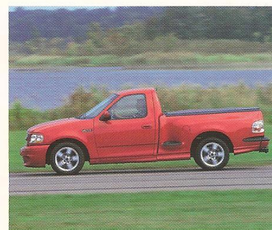
2001-2002 SVT F-150 Lightning 5.4L SOHC supercharged V-8 380 horsepower 450 ft-lbs of torque Production: 11,107 units
