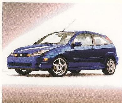
2002 SVT Focus 2.0L DOHC I-4 170 horsepower 145 ft-lbs of torque Production: 4,788 units
