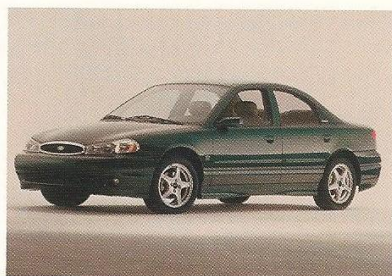
1999-2000 SVT Contour 2.5L DOHC V-6 200 horsepower 169 ft-lbs of torque Production: 4,910 units
