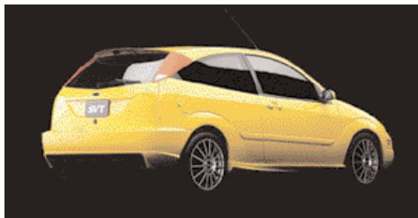
Rocker moldings, hatch spoiler and rear fascia set the SVT Focus apart.
