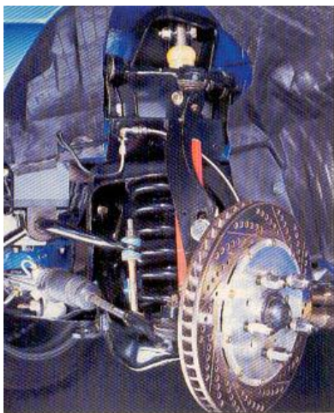
Ultimate go requires premium, racing-style four-wheel-disc stopping muscle. Squeezing the whoa pedal activates anti-lock-controlled eight-piston, four-pad Brembo calipers in front and four-piston, two-pad calipers in the rear. The 13-inch front rotors are cross-drilled and slotted. In back are 12-inch cross-drilled discs.
