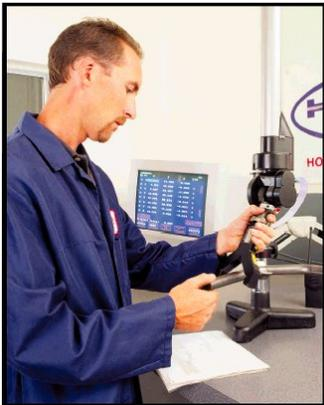
computer keeps track of each bend in relation to all of the other bends. This produces a very high tolerance part, typically in the 0.050" range or tighter, and with consistent reliability. During the manufacturing run, a Laser Vector inspection system is employed to measure the parts being bent by the machine. This measures the shape of the bar, and compares it to a computer file of the part print. The laser's computer sends any necessary corrections directly to the bending
