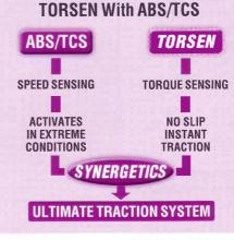
The TORSEN Traction Differential is a rugged clutch-free system that works instantly. There is no lag time or wheel slip as in old LSD technology. In addition, it is a full-time, continuous-duty unit, bearing the brunt of the traction management work while ABS/TCS kick in only under extreme conditions. Each system enhances the other, providing increased longevity, assuring continuous and reliable long-term performance.
