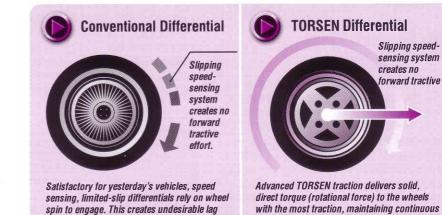
direct torque (rotational force) to the wheels with the most traction, maintaining continuous control for better vehicle performance.
